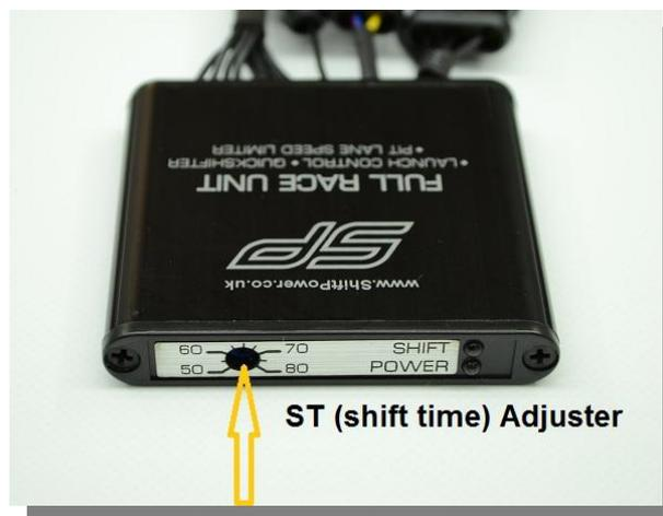
➤ ST(Shift Time) adjusts the engine interrupt time for which the gearbox must engage the next gear after you apply enough pressure to the gear lever:... turn it clockwise for more time or anticlockwise for less time. The adjuster starts from 50ms(milliseconds ), each setting is recognized by a light code on the blue “SHIFT” light. Light codes are implemented to ensure exact settings are selected. The following table shows the time settings with the corresponding light codes:
